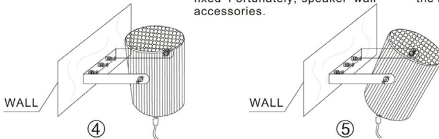
4. Figure, a 90-degree vertical installation in the wall fixed. Such as the need to change the point of view can be moved to install speakers.
