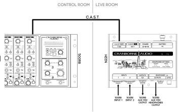
DC power supply or via an internal 9v battery. Power is only drawn when the headphone output has been plugged-in to preserve battery life and when the headphone amp is not required, you can simply use the combi jack inputs as passive input connections.
