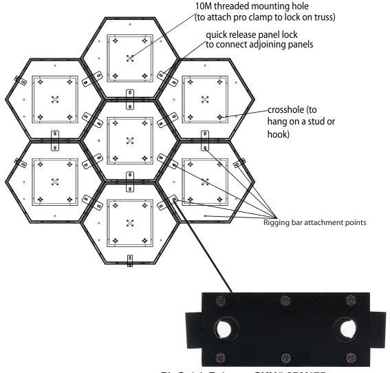
PL Quick Release: **SKU# 3DV175**Quick Release panel lock is used to connect the units to one another. See page 15.
