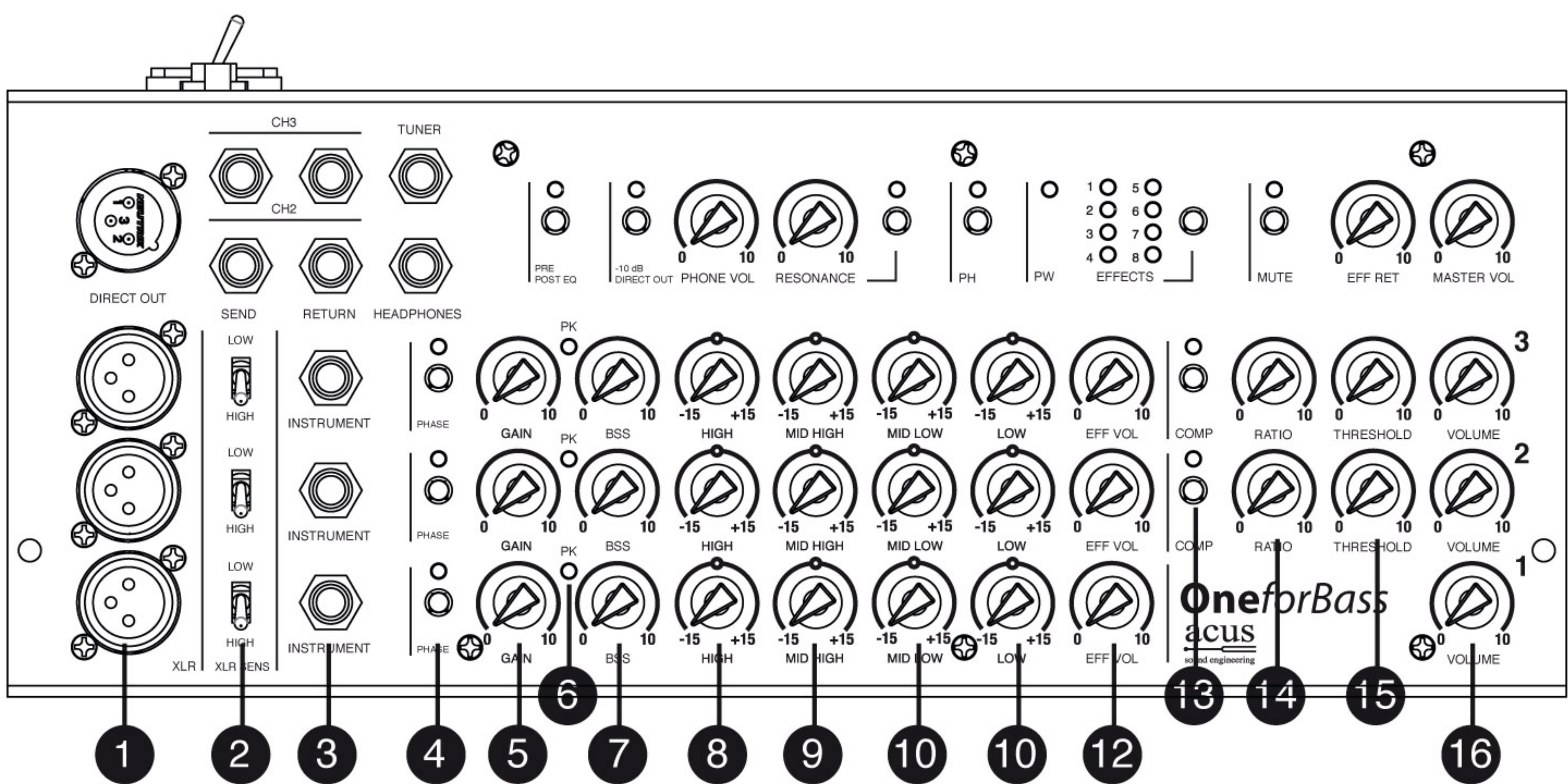
**1-XLR:** Balanced input. It can be both line input and microphonic input.
