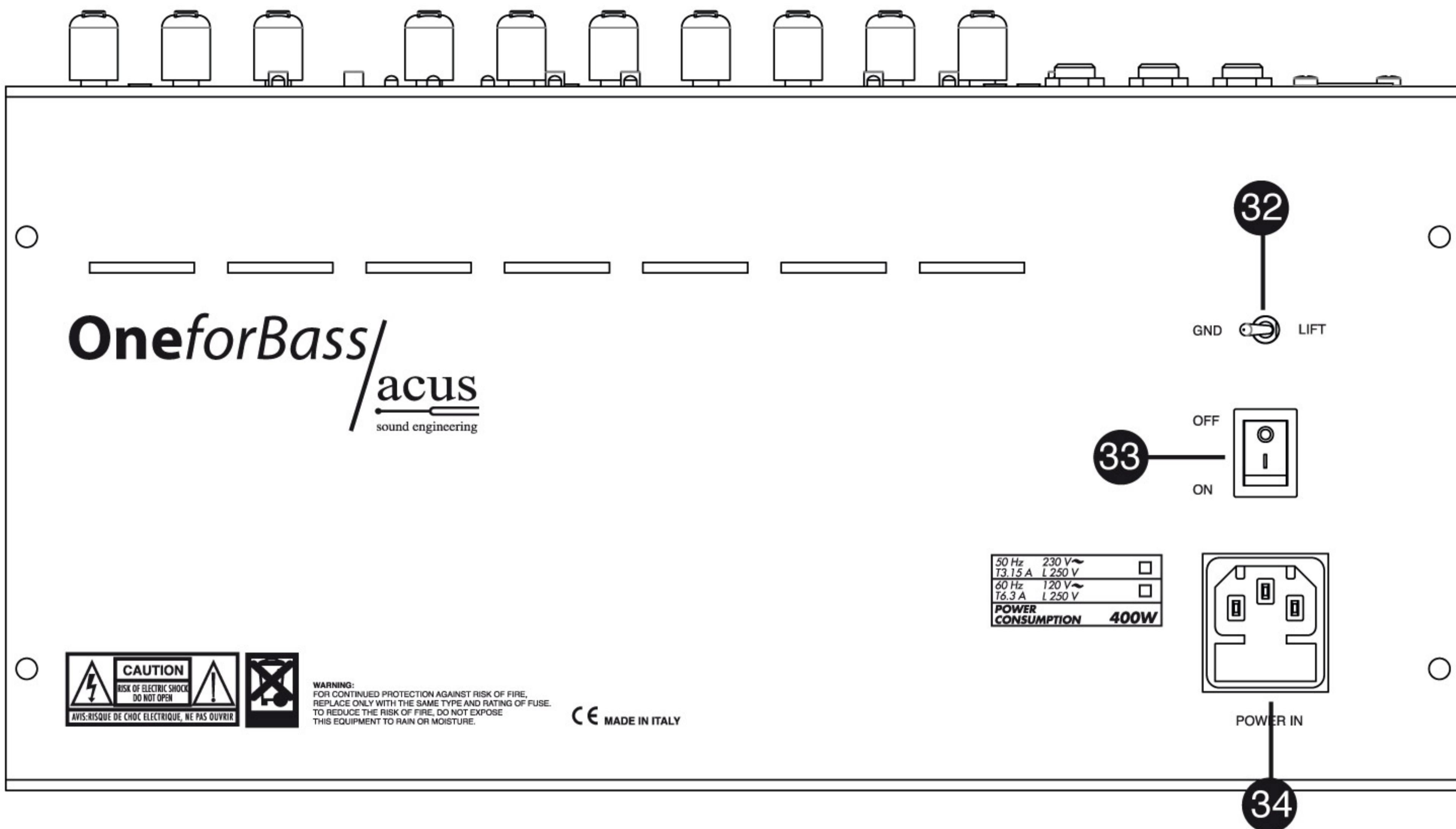
**32-GND LIFT:** switch grounding of the electronic circuit. Revert the position in the event of a humming noise generated by the power supply.
