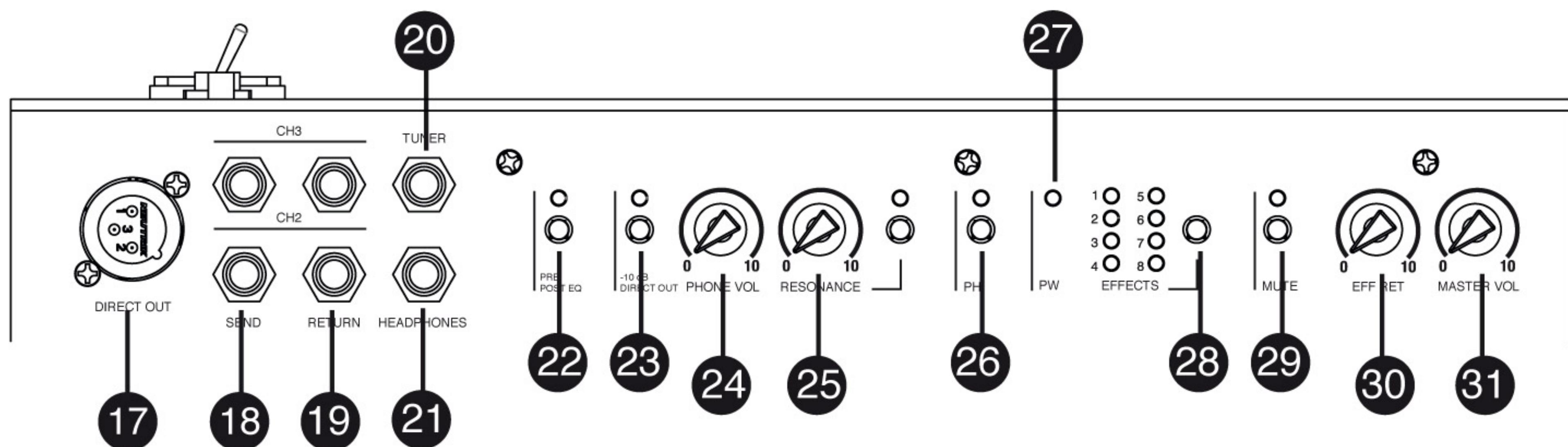
**17-DIRECT OUT:** Balanced output. Its level is independent from the Master Volume but it is a function of the -10dB Direct Out switch position.
