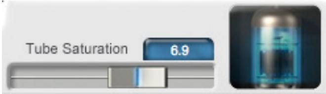
The Tube Saturation section is based on Antares' renowned WARM Tube Saturation Generator and is designed to model the "warmth" that is typical of a high-quality tube pre-amp.
