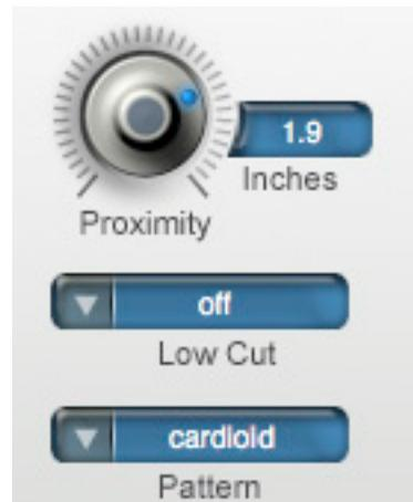
If the mic you select in the Modeled Mic menu is equipped with a user-selectable low-cut filter, the Low-Cut pop-up menu will allow you to select from among the filter settings available on that mic. (If the selected mic does not have a low-cut filter, the menu will be grayed out.)
