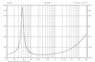
CH A Ohm Resolution 1/48 Octave Unsmoothed Delay [ms] 0.000 Dist Rise [dB] 30.00
