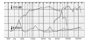
BMS 4595-8, incl. passive crossover, 2nd + 3rd harmonic distortion raised 10dB., SPL 1W / 1m
