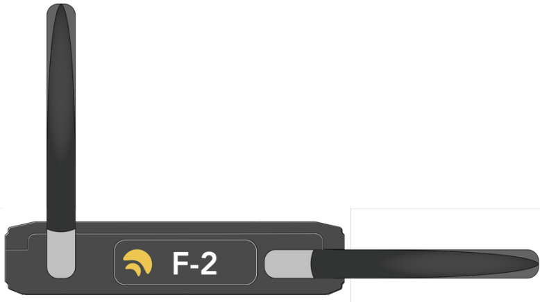
Fig.3: It's possible to increase performance of dual-universe devices just by rotating one of the antennas to a different axis. This will avoid the radio-waves of both transmissions to interfere with each other.
