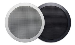
The Apart CM6E is a dual cone 100 volt / 8 ohm built-in ceiling loudspeaker. The loudspeaker has a 6.5" dual cone woofer and a high quality 100 volt speaker line transformer with multiple power taps. CM6E is the perfect choice for the distribution of microphone calls and background music. The mounting frame is made of high quality ABS. CM6E is available in black and white.
