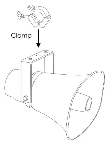
The HS-30S can be mounted to any kind of truss with a clamp.
