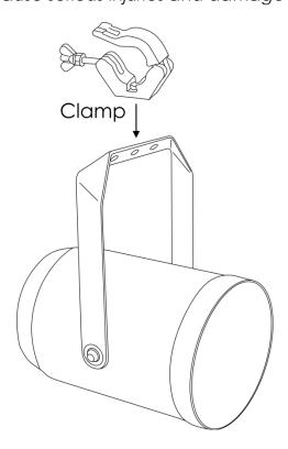
The PSU-510P can be mounted to any kind of truss with a clamp.
