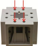
2. Now turn the WMS bracket and remove the front and back lid as shown in figure 3.
