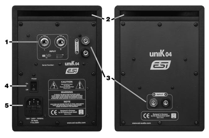
**1. TRS input (Left / Right)** – these jacks accept TRS input connections, either balanced or unbalanced. For balanced connections, a 3-conductor TRS plug is necessary. The TRS input is wired like this:
