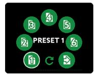
After selecting the desired preset by using the SE-LECT pot and MENU to load it a second screen appears. This screen lets you choose what should be loaded: The GAINS of the analog inputs, the LEVELS of the analog outputs, the routing – or all three items. To store a current setting into a preset slot, enter the STORE menu:
