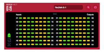
The illustration above shows a RedNet 6, with signal present on every channel and a locked network connection with SRC's turned off.
