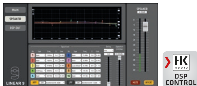
Screenshot of the remote DSP CONTROL software. You can download this software free of charge at the LINEAR 9 product page at www.hkaudio.com . The speaker and DSP Out parameters are identical, but the powerful onboard DSP lets you configure each set independently.
