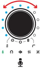
When the microphone symbol is lit **green**, the knob will control the microphone gain and the LED ring will show the peak level of the microphone's capsule signal.
