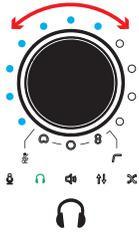
When the headphone symbol is lit **green**, the knob will control the level of the headphone output and the LED ring will show the peak level of the overall streamed signal.
