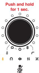
By pushing and holding the knob for 1 second, the signal of the microphone's capsules will be muted. When the mic is muted, the microphone symbol will blink **orange**. The LED ring will continue to show the peak level of the overall streamed signal with the same logic described above.
