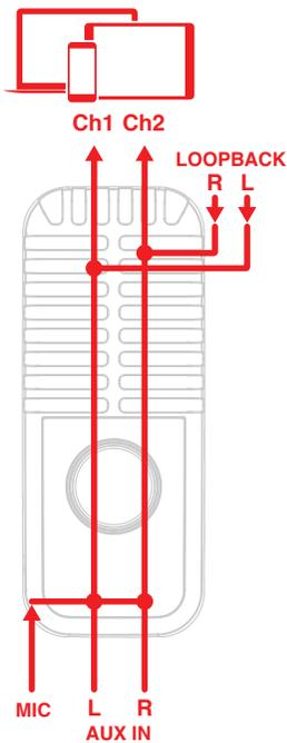
The microphone capsules routing depends on how the polar pattern is set: mono (cardioid, omni and fig.8) or stereo. When the stereo pattern is selected, MIC front capsule is routed to CH 1 and MIC back capsule is routed to CH 2.
