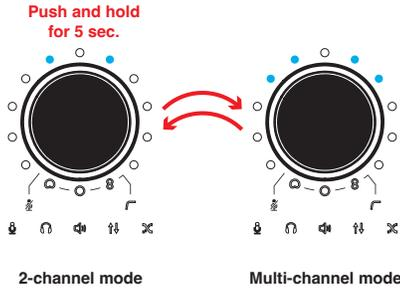
By pushing and holding the knob for 5 seconds the device will enter the operation mode menu. The LED ring will show the current mode selected (2-channel or multichannel).
