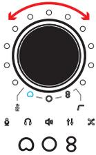
When one of the pattern symbols is blinking blue, you can select the polar patterns by rotating the knob and the LED ring will show the peak level of the overall streamed signal.
