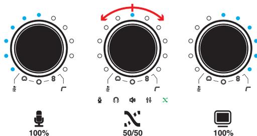
When the monitor mix symbol is lit **green**, you can adjust the mix between the microphone signal and the sound from the connected host in your headphones.
