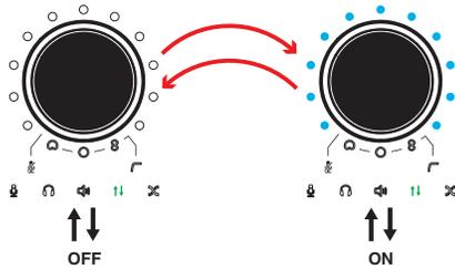
When the loopback symbol is lit **green**, you can turn on or off the loopback feature by rotating the knob: CW rotation will activate the loopback and the LED ring will turn on, CCW rotation will deactivate the loopback and the LED ring will turn off.
