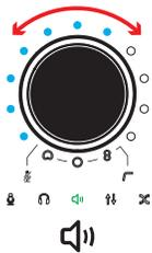
When the streaming symbol is lit **green**, the knob will control the level of the overall streaming signal (capsules, aux in and loopback) and the LED ring will show the peak level of the overall streamed signal.
