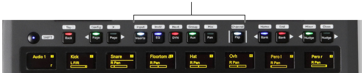
Channel Encoder Assign switches (showing all switches lit to indicate primary LED colors)
