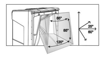
The acoustical design allows to face different environments. The dispersion pattern is asymmetrical on the vertical axis, and the horizontal coverage varies within position: It is wider in the lower side and narrow in the upper one.
