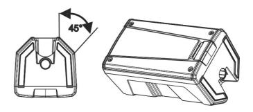
The rear side inclination, symmetrical, as shown in the upper picture, is 45°. The related wedge positioning is shown in the picture. B-HYPE can be used as a stage monitor in small contexts, in this case please consider the characteristic dispersion pattern presented above.
