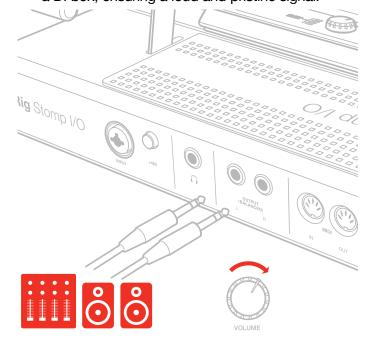
6. Connect your headphones to the headphone output. It is possible to control the output volume with the Volume potentiometer on the top panel.
