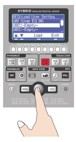
To return to the previous screen without recalling equalizer settings, press the EXIT button or the function button indicated as "Exit."
