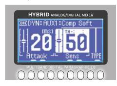
Press the white button under the word **TYPE** on the LCD screen.
