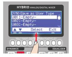
Scroll up or down with ▼ and ▲, or the encoder knob, pick an *Empty* location and press *Select*.
