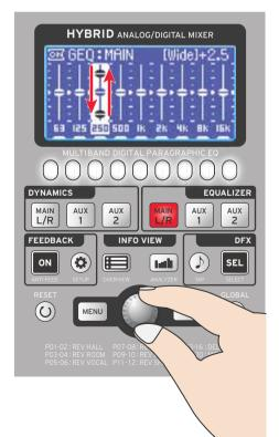
9 Press down on the encoder knob to return to the 31 / 9 (*Narrow*) EQ mode and view the results of your adjustment.
