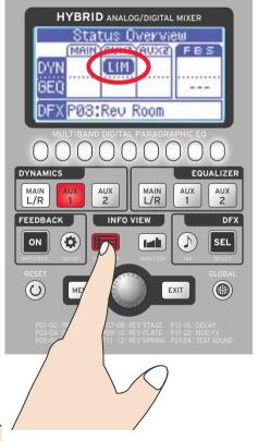
8 How do you cancel a dynamic processor? Press the active (designated blinking) **DYNAMICS** button. The effect with stop, the
