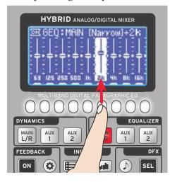
**Push down** on the encoder knob to change the screen to 31/9 (Narrow) EQ mode.
