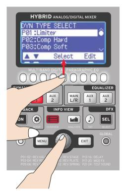
To select a dynamic effect (in our example, Limiter), press and hold the button under Select OR push down on the encoder wheel until you feel a click.
