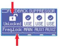
Press the function button indicated as "Freq.Lock" to switch the setting between "Locked" (locked) and "Unlocked" (not locked).
