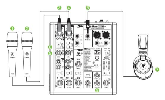
The two **EM-89D** Microphones ① ② are connected to channels 1 and 2 ③ ④ on the **ProFXv3** mixer. Set the Gain control ⑤ so that the Level Set LED for each channel lights up whenever the source (your voice, drums, guitar, etc.) hits its average volume level.
