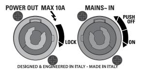
MAINS IN - Powercon® NAC3FCA power input connector (blue). To switch the amplifier on, insert the Powercon® connector and turn it in a clockwise direction into the ON position. To switch the amplifier off, pull back the switch on the connector and turn the connector in an anticlockwise direction into the POWER OFF position.
