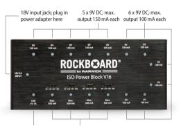
USB 5V; max. 4 x switchable slots with 9V DC / 12V DC / 15V DC / 18V DC; output 1 A each max. output 300 mA at 9V, 200 mA at 12V, 180 mA at 15V, 150 mA at 18V
