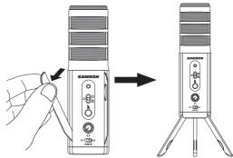
Set the Satellite's pattern switch. If you are recording a single person, set the switch to the Cardioid position and be sure to face the front side, with the Samson logo. If recording two people, set the microphone to the Bidirectional position and if recording multiple subjects, set the switch to the Omnidirectional position.
