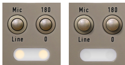
Input & polarity indicator lamps and their button positions. At left: Mic input selected and inverted Polarity. At right: Line input selected and normal Polarity.
