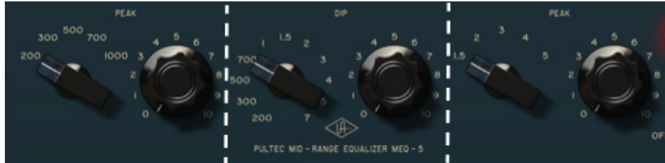
Control grouping within the Pultec MEQ-5
