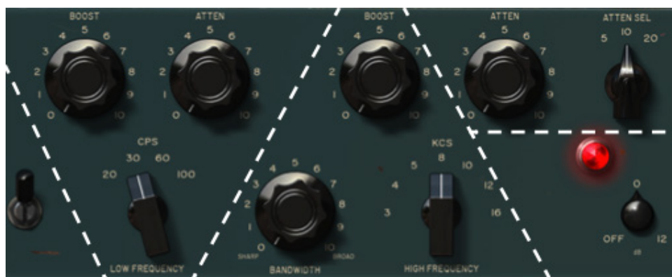
Control grouping within the Pultec EQP-1A
