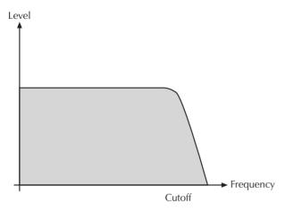
To give you an idea of the extent of damping, consider this example of a lowpass filter: a reduction of 24dB reduces the original level one octave above the cutoff point by approx. 94%. The damping factor two octaves above the cutoff point reduces the original level by more than 99%, which in most cases means this portion of the signal is no longer audible.
