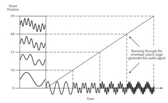
hen you play a note, the envelope advances the position through the wavetable, generating different waveforms over time.
