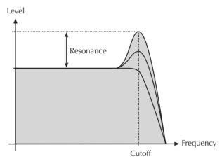
If the resonance is raised to a great extent then the filter will begin self-oscillation – i.e. the filter generates an audible sine wave even when it does not receive an incoming signal.
