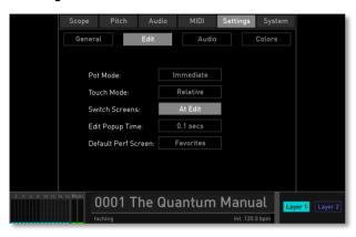
• Pot Mode: tap on this button to select the behaviour of the potentiometers (not the endless dials). *Immediate* means that a parameter value will jump immediately to the corresponding dial position. *Pick-Up* means that you have to turn the dial until it reaches the current parameter value. If reached, the value is changed. *Catch* works almost the same as Pick-Up, but the current value moves while turning until the dial position matches the value.
