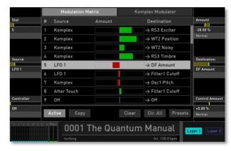
This page shows all modulation assignments in a list. You can set up to 40 assignments.
