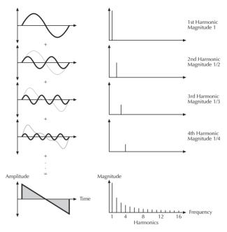
Additive components of the Sawtooth wave
