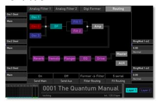
Here you see a graphic overview of the Quantum's signal routing. You can also control the routing of the three oscillators, ring modulators, and set up the audio outputs for the current sound.
