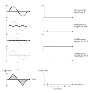
Additive components of the Triangle wave
