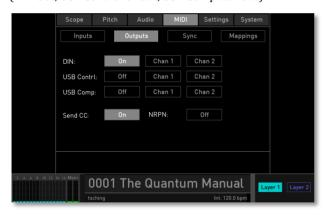
State: Tap on this button to switch the corresponding MIDI Out on or off. Keep in mind that the arpeggiator
