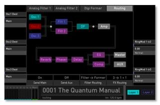
Potential signal routing for an audio signal
