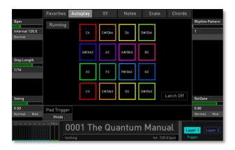
If no pad is latched all display pads will be used to sequence the notes. For rhythmic variation you can use the parameters **Rhythm Pattern**, **Swing** and **Rel Gate**.
