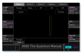
For the typical Flanger effect sound the **Dry/Wet** parameter should be set to 50%.
