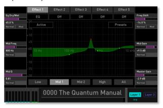
Tap on the corresponding EQ curve in the touchscreen display to edit the **Frequency** and **Gain** parameters.
