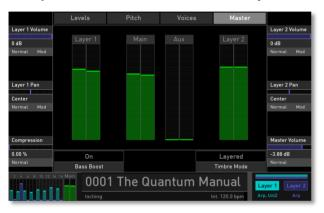
The current volume of Layer 1, 2 as well as Main and Aux volume is displayed in the gain meter representation.
