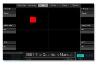
First you need to define the X and Y controllers within the **Modulation Matrix**. You can, for example, easily set up a modulation for Cutoff (Pad X) and Resonance (Pad Y).
