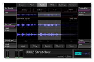
The Audio tab display with Input as Recording Source
