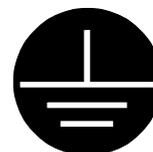
For safety it is important that all equipment earths are connected to mains earth so that exposed metal parts are prevented from carrying high voltage which can injure or even kill the operator. It is recommended that the system engineer check the continuity of the safety earth from all points in the system including microphone bodies, turntable chassis, equipment cases, and so on.
