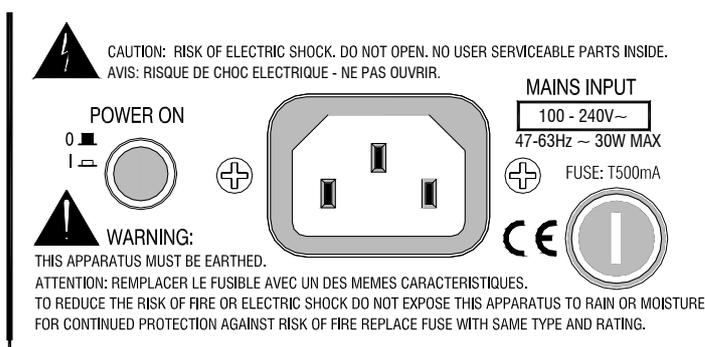
**Connecting Mains Power** Read the SAFETY INSTRUCTIONS printed at the front of this User Guide and on the rear panel. Check that the correct mains lead with moulded plug has been supplied with your console. The power supply accepts 50/60Hz AC mains voltages within the range 100-240V without changing any fuses or settings.
