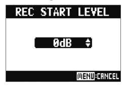
Recording will start automatically when the level of the MASTER fader output signal exceeds the set level.
