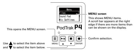
In this Quick Guide, MENU item names are shown with gray backgrounds, and the procedure of selecting items on the MENU screen using [n], [n] and [n] is abbreviated as follows.
